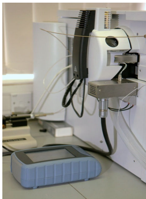
Ultra-FAIMS microchip installed on Agilent 6230 TOF
