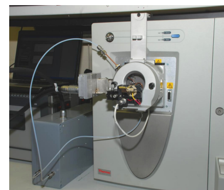
Fig. 3. (right) Photo of the FAIMS device mounted in the nanospray housing. Fig. 4. (left) photo of the entire add-on system integrated on to the Thermo LXQ
