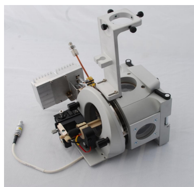
Fig. 3. (right) Photo of the FAIMS device mounted in the nanospray housing. Fig. 4. (left) photo of the entire add-on system integrated on to the Thermo LXQ
